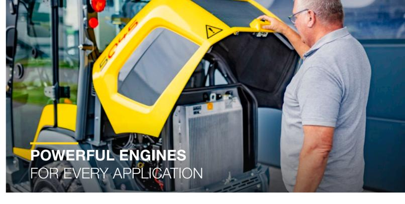
The 5035 and 5045 are driven by a Yanmar 18.5 kW engine without exhaust after-treatment. The 5040 is equipped with a Yanmar 28.5 kW engine. The 5045 is optionally available with a Yanmar 33.5 kW engine. The exhaust after-treatments on both engines are with DOC and DPF.
