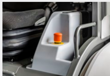
Quickly accessible emergency switch, so that the machine can be immediately transferred to a safe state in an emergency.
