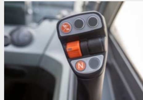
Comfortable joystick: Possible to switch between the tortoise and the hare directly on the joystick.
