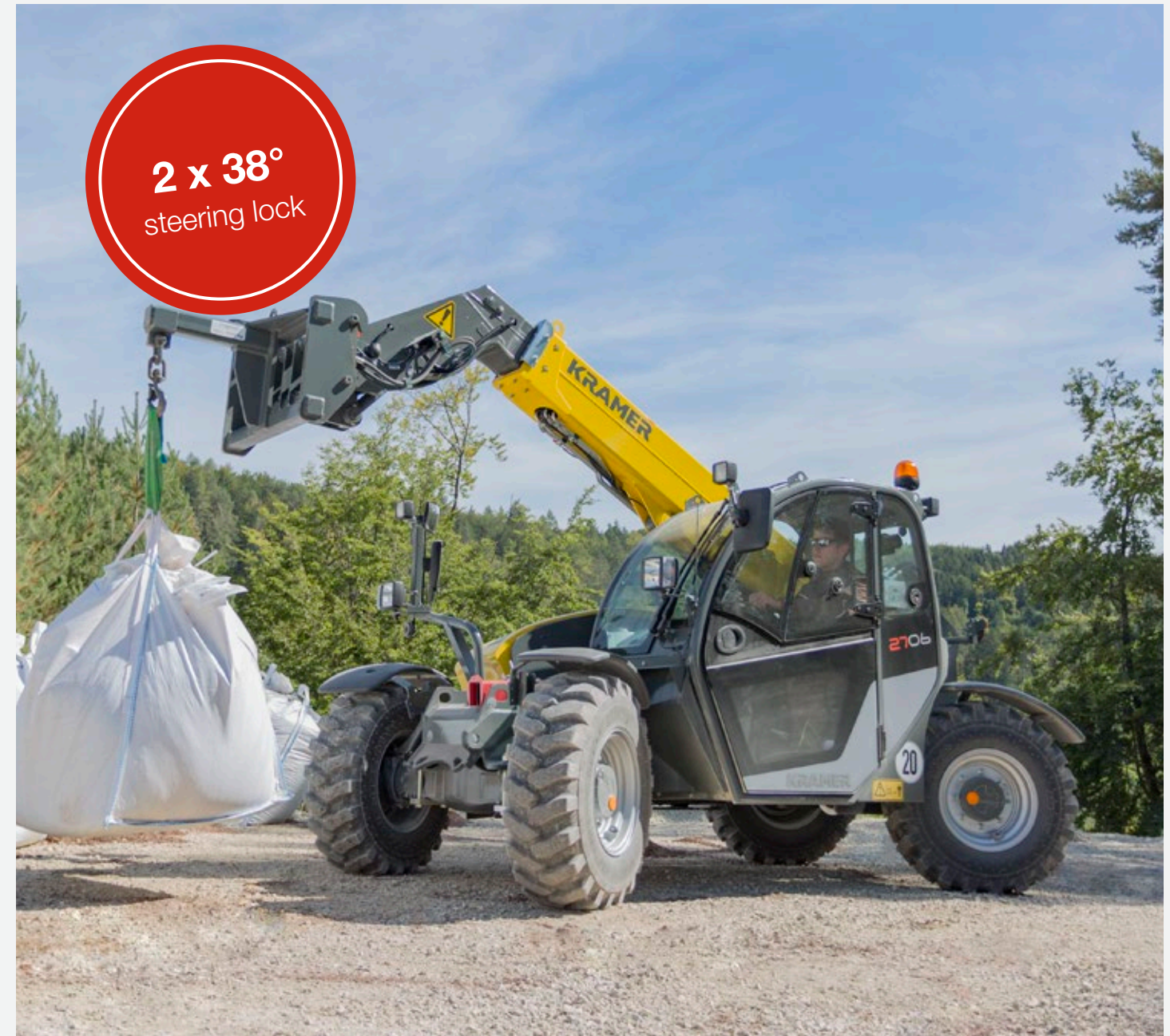
All-wheel steering: particularly manoeuvrable in tight spaces
