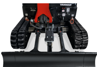
Extended undercarriage: 1170 mm
