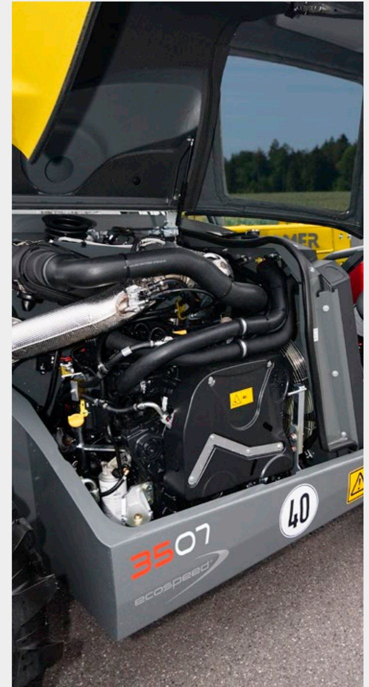
Water-cooled 4-cylinder in-line engine with cooled external Exhaust gas recirculation, turbocharging and intercooling.
