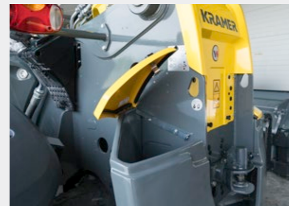
Storage compartment in the rear weights for 4507 - 5509
