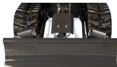
Retracted undercarriage : 955 mm
