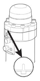
Install the back head onto cylinder housing where the marks meet each other.
