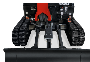
Extended undercarriage: 1 380 mm
