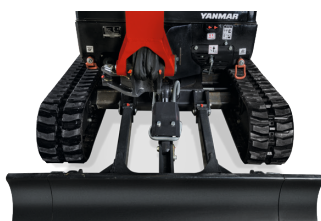
Extended undercarriage: 1170 mm
