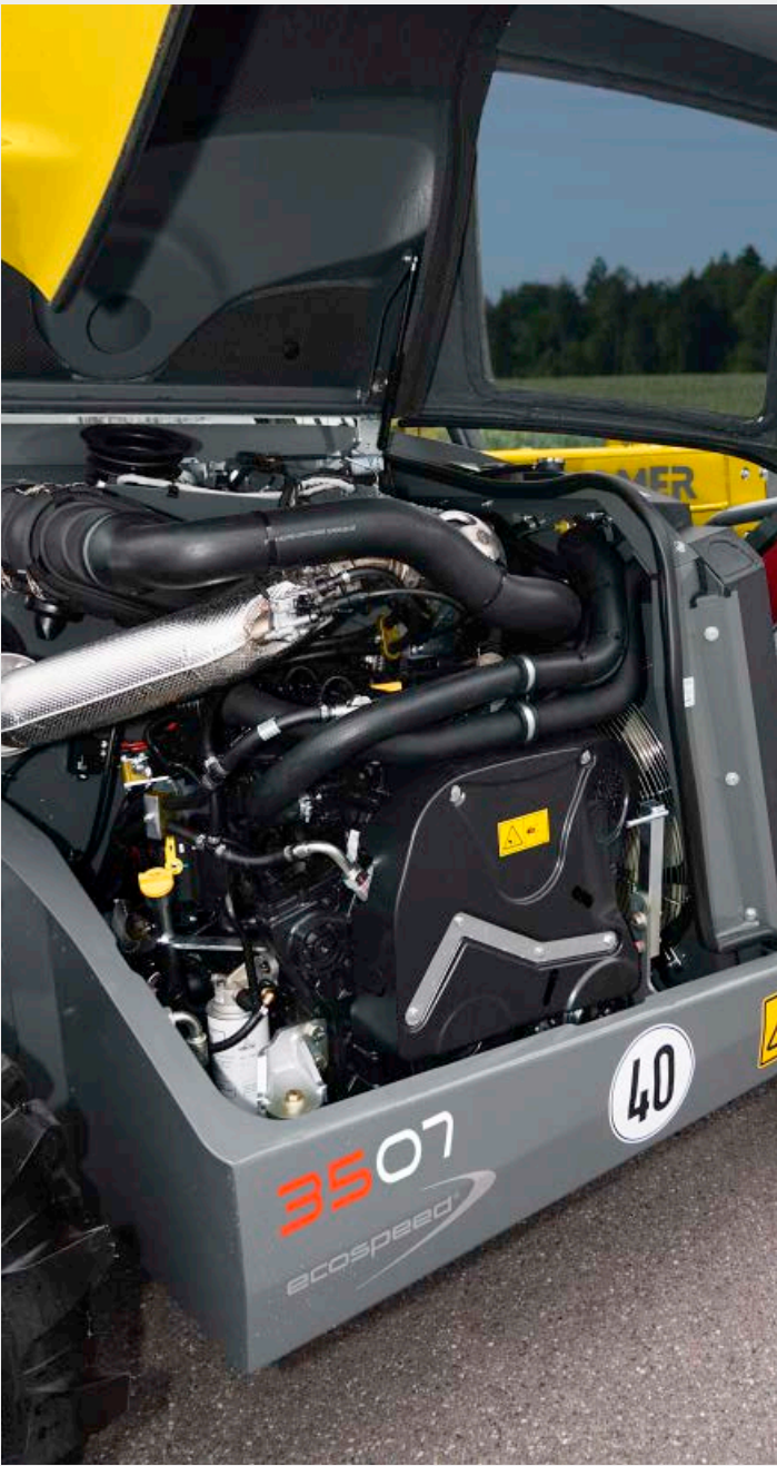
Water-cooled 4-cylinder in-line engine with cooled external Exhaust gas recirculation, turbocharging and intercooling.
