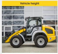
The machines offer the best conditions for low headrooms. All machines have an overall height of less than 2.5 m. The compact construction of the wheel loader 5050 enables easy transport on a 3.5 t trailer.
