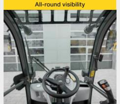
The central seat position of the operator offers a 360° all-round visibility. "Blind spots" are avoided thanks to the particularly clearly arranged design. You can even see everything to the rear. Even when the telehandler system is extended on the 5065T, the operator has a perfect view of the attachment.
