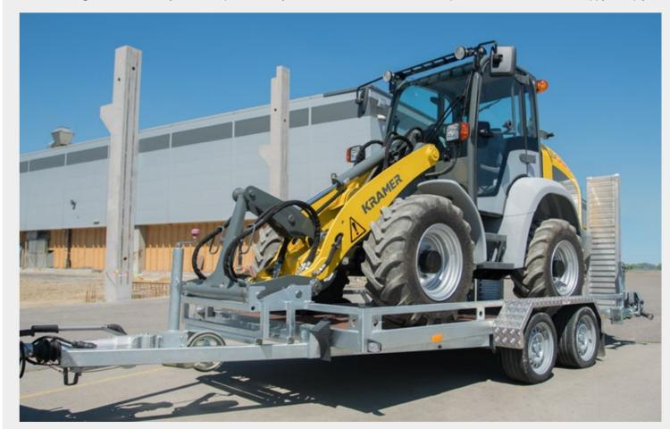
Quick and easy load securing by locking directly to the trailer with the Kramerquick coupler system seating.
