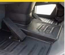
The central terminal in the cabin floor is just 5cm high, due to the design of vehicle frame. This therefore enables the operator to get in and out easily. The central tunnel is also covered with a rubber mat which is easy to clean.
