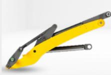
Specific customer wishes can be met even more flexibly due to the extended loader unit. Among other things, the range, payload and lift height change compared to the standard loader unit.
