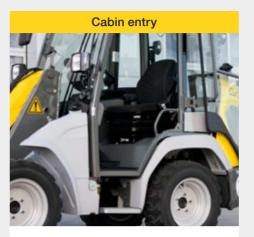
The wide entry includes additional steps, thus ensuring comfortable entry and exit. Two grab handles fixed to the cabin help the operator to get in and out of the cabin safely. The cabin door can also be opened through 180 degrees and locked to the machine.
