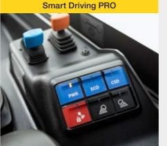
The feature with the 5040 includes three different drive modes that can be changed at the push of a button, to confront any requirement with the greatest efficiency. The power mode (PWR) is ideal for bucket work, the ECO mode the stacking work or road travel and the low-speed control (CSD) for hydraulic attachments.
